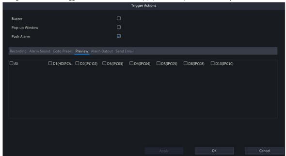
The live view page displayed in the event of alarms varies depending on the number of linked cameras and the number of alarm-triggered live view windows. When an alarm occurs, the live view page shows the live video from the linked camera(s) with a red frame; when the alarm ends, the live view page returns to the original state.
