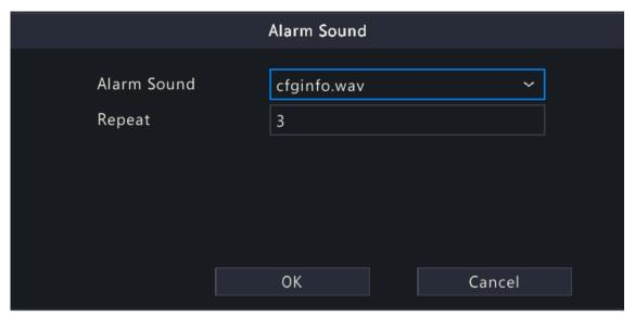
2. Select the desired IP speaker(s), enable alarm sound, and click **OK**.
