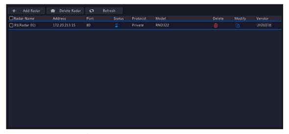
2. Click Add Radar, and then configure radar parameters.
