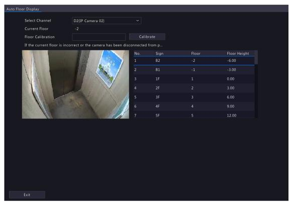
3. If the displayed floor is incorrect, input the correct floor, and then click Calibrate to correct it.
