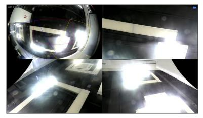
• Drag the mouse to rotate the image or use the scroll wheel to zoom in or out on a PTZ image. A box appears on the fisheye image as the image rotates, and as you drag the box or move the scroll wheel on the fisheye image, the corresponding PTZ image rotates or zooms in or out as well.
