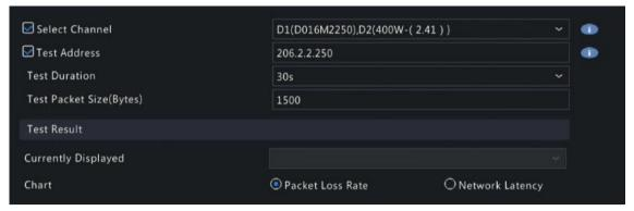
6. Click **Test** to test the packet loss rate and network latency.
