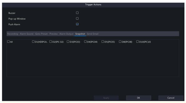
Note: This action is only available to certain alarm functions such as motion detection and human body detection, and is not available to VCA functions.
