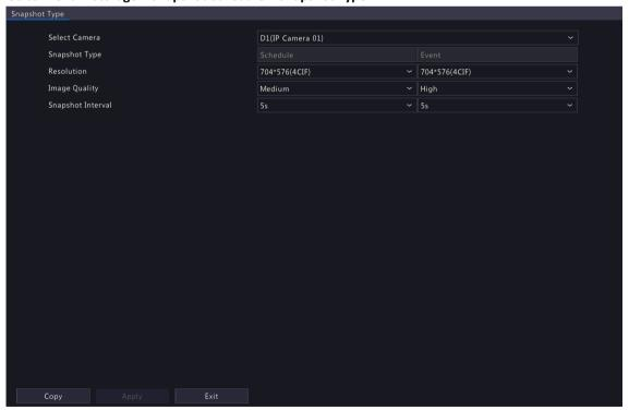
2. Select the camera and set the parameters as needed.
