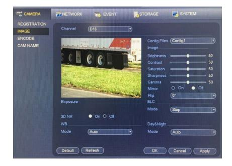
If you plan on capturing license plates at night you may need to Adjust the Day/Night mode from Auto to Colorful. This will enable the camera to stay in a color mode at night. This drops the IR night vision intensity and will prevent License plate reflection at night.
