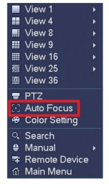
Inside of the Auto Focus menu you may click and hold the click down on the slider. Move the mouse left and right to drag the slider to make adjustments to the zoom. Once the camera zooms in, give it enough time to Auto Focus. Once the camera is Auto Focused you will be able to control it again.
