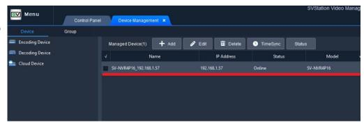
Now that our device has been added into SVStation we can now exit the Device Management section. This workstation is now ready to view the your cameras!
