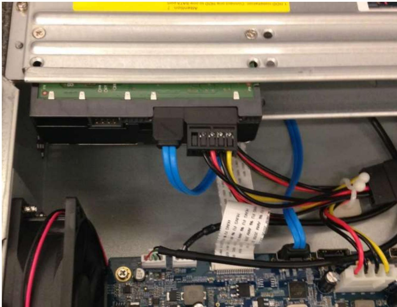
Once the hard drive is mounted and connected you may assemble the top cover and fasten the four case screws removed previously in the guide.
