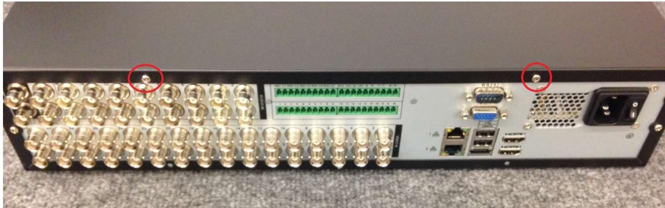
Once these screws have been removed the top cover will slide towards the rear and lift off.
