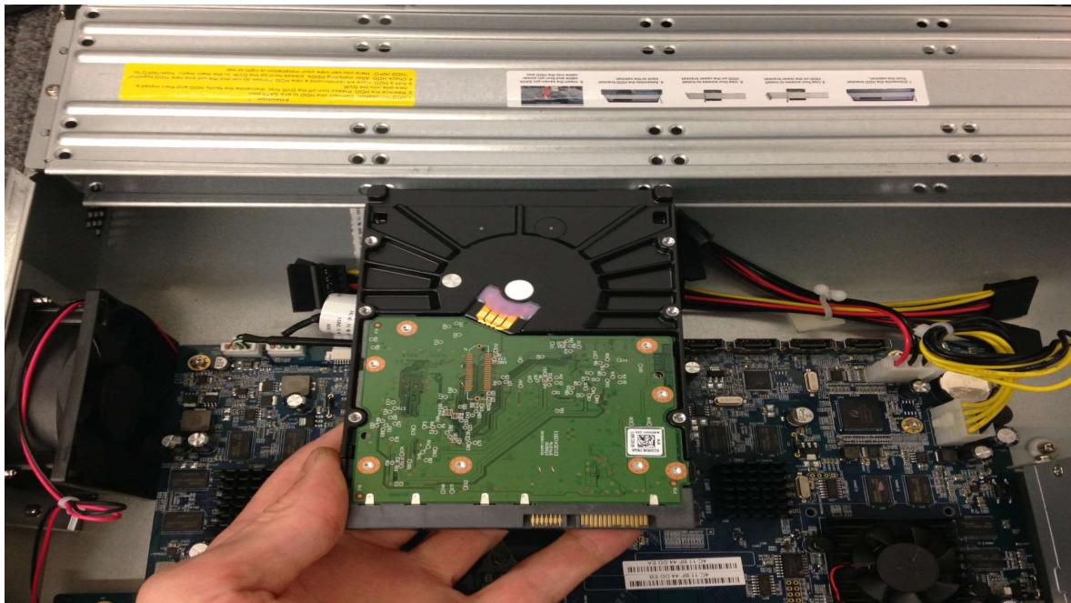
You can now mount the Hard Drive to the Chassis using the supplied screws.
