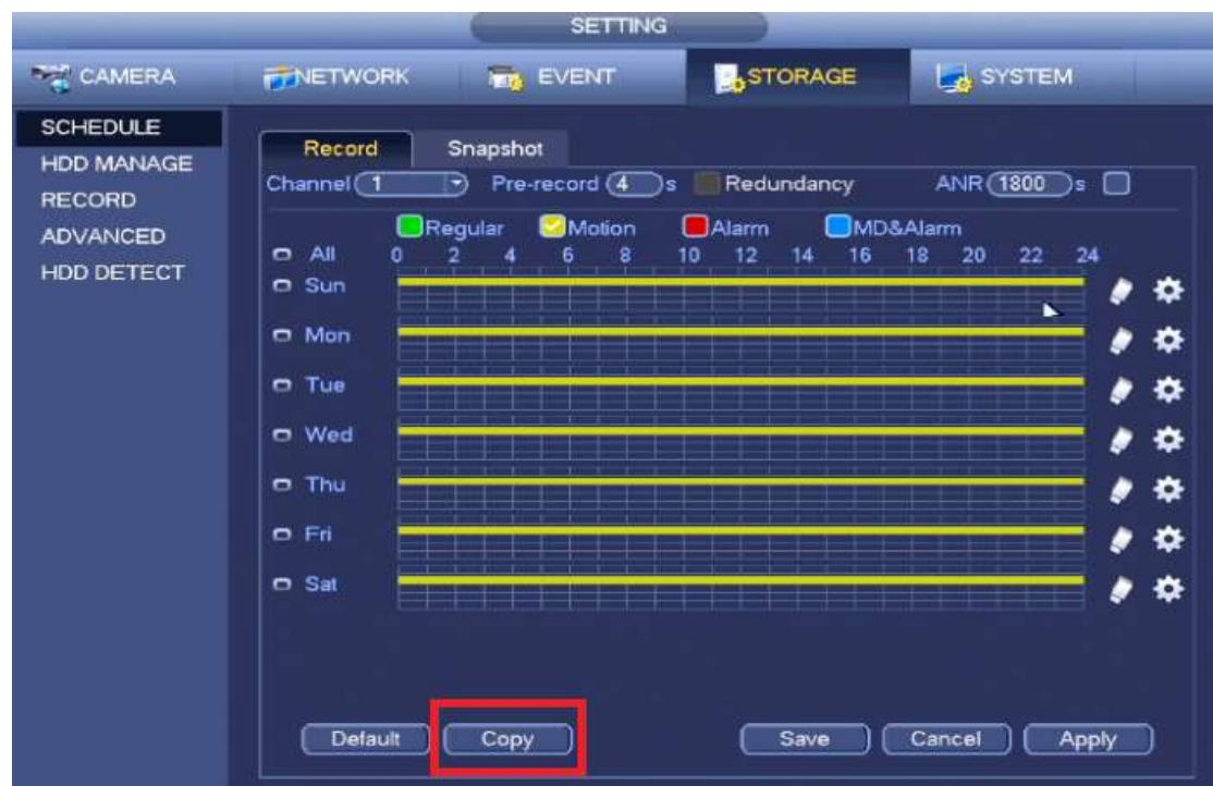
We have now successfully setup a **Motion Detection Schedule**. We now want to make sure Motion Detection is **Enabled** for each Channel. This can be done by going back to the **Main Menu** → **Setting** → **Event**
