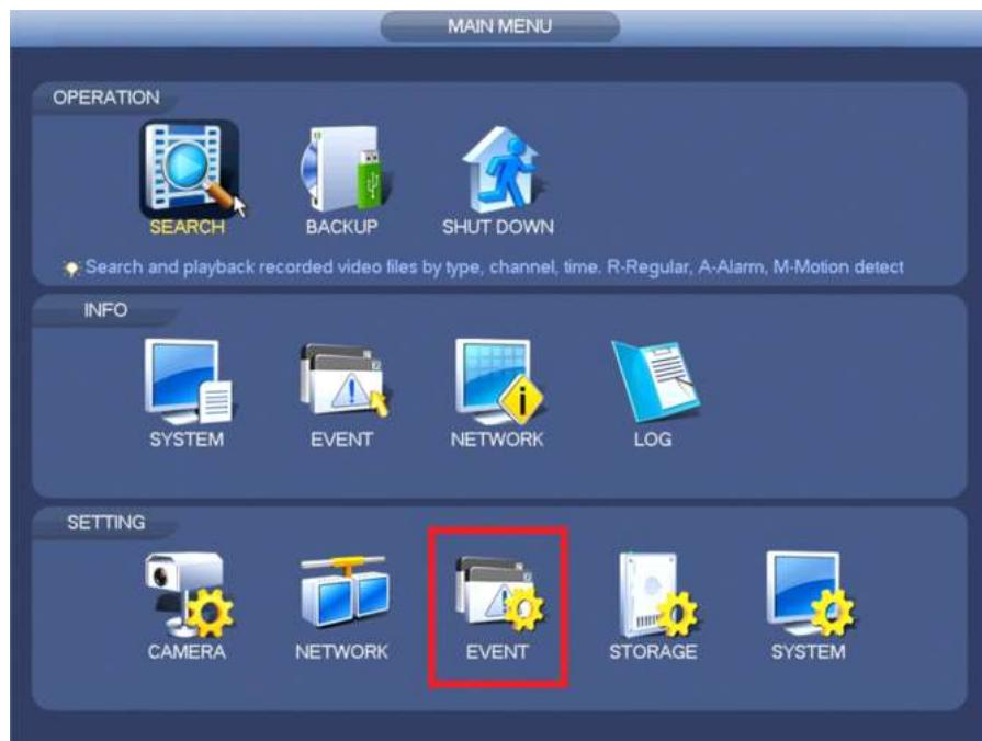
Inside of the **Event Settings** Click on **Video Detect**. Make sure to check each Channel number and Click the **Enable** Check Box. Do this one Channel at a time. **NOTE: Do not use the Copy button on this menu!** **Apply** and **Save** once all Channels have been enabled.
