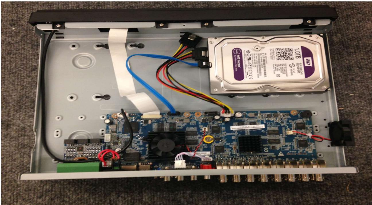
You can now turn the DVR over and mount the Hard Drive to the Chassis using the supplied screws.
