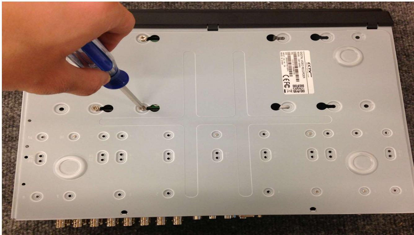
Once the hard drive is mounted you may assemble the top cover and fasten the four case screws removed previously in the guide.
