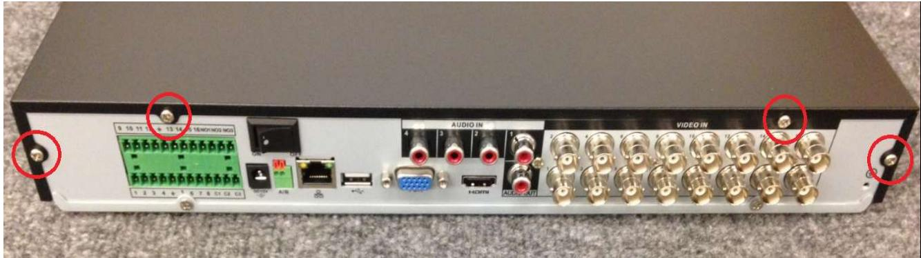
Once these screws have been removed the top cover will slide towards the rear and lift off.
