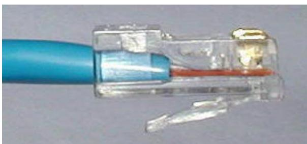
Carefully push all 8 colored wires into the connector. Note the position of the blue plastic sleeve. Also note how the wires go all the way to the end.
