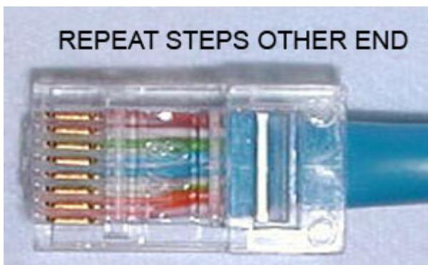
For a standard "Straight Through" cable, repeat all steps and wire color order on the other end of cable.
