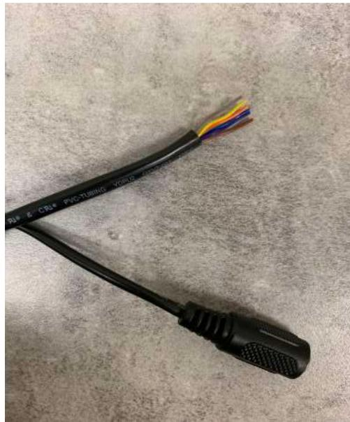
Organize the cables to match the pinout of the IP camera. Slide the organized cables into the connector and crimp. All CCTV Security Pros IP cameras will use this pinout.
