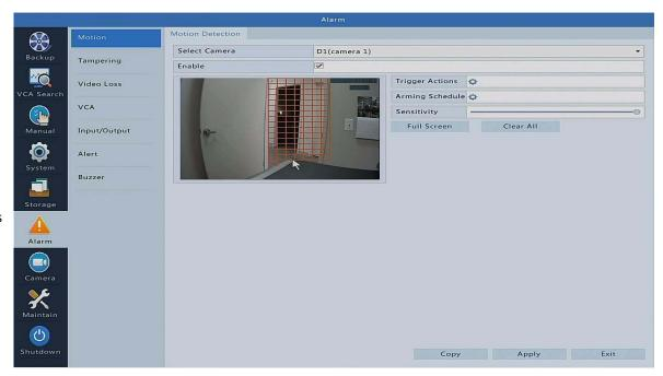
You may adjust the motion detection Sensitivity using the slider bar. The higher the number the more sensitive the motion will be. The lower the number the less recordings you will have. There are a few different options to check out in this menu as well such as Trigger Action and Arming Schedule, these are explained below.
