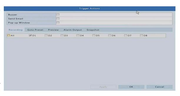
We recommend keeping the **Recording settings** at the bottom set to default. Altering this may record the incorrect camera when motion is detected.
