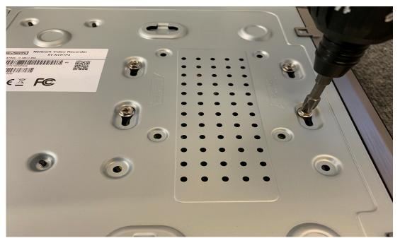
Once the hard drive is mounted you may assemble the top cover and fasten the four case screws removed previously in the guide.
