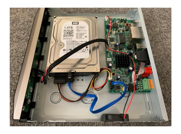
You can now turn the DVR over and mount the Hard Drive to the Chassis using the supplied screws.
