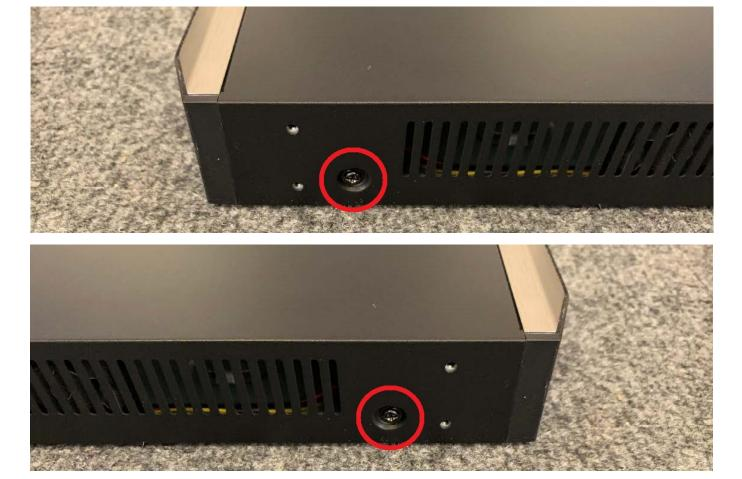
Once these screws have been removed the top cover will lift from the rear and slide off.
