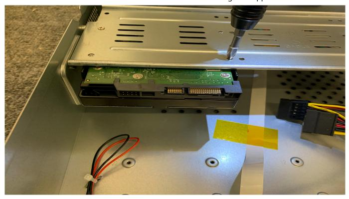
Connect both the Blue SATA cable as well as the SATA Power cable. This cable will be found installed already in your NVR.
