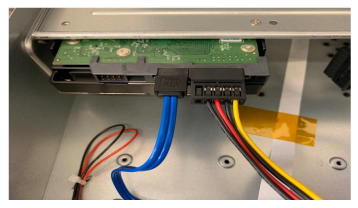
Once the hard drive is mounted and connected you may assemble the top cover and fasten the two screws removed previously in the guide.
